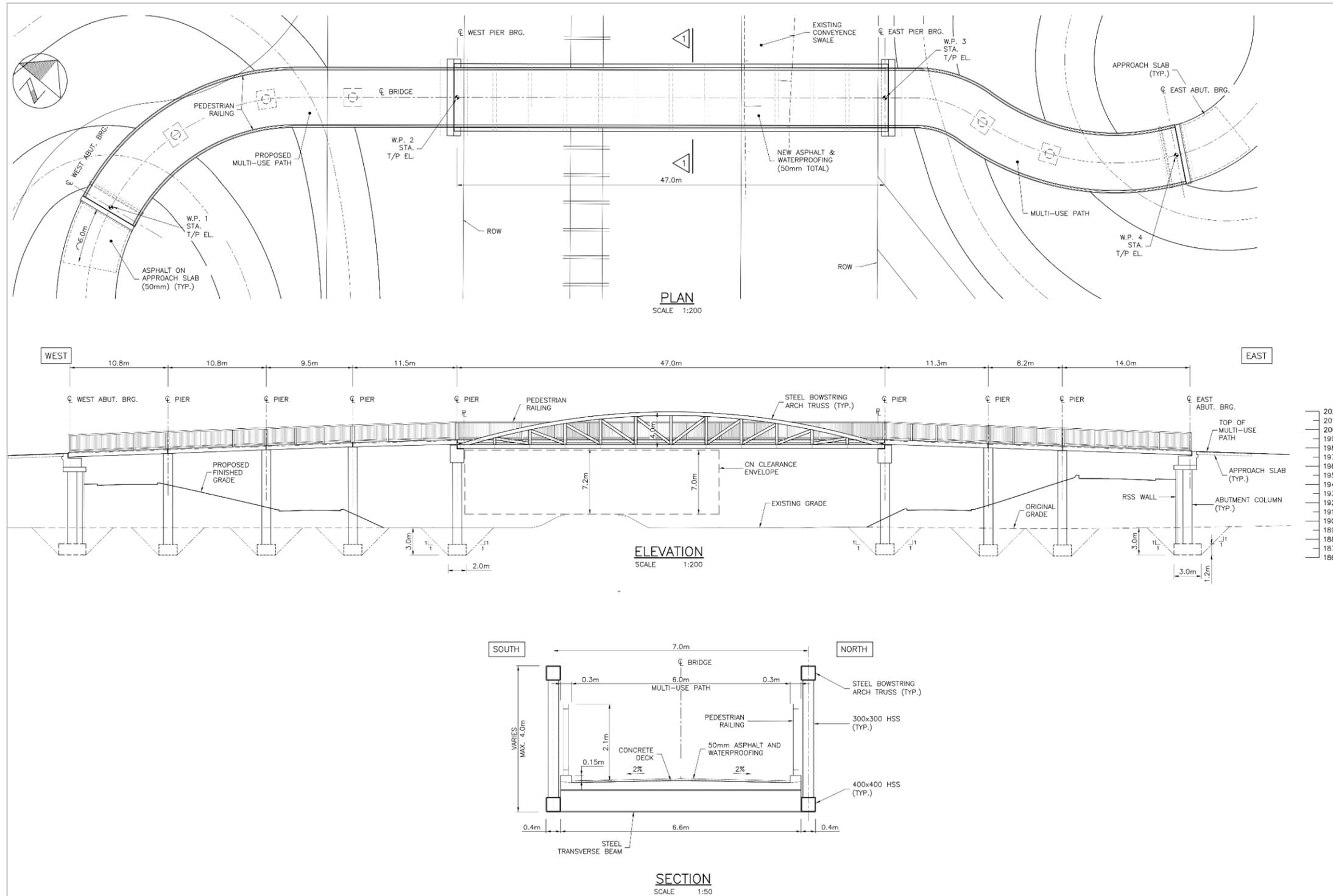
Figure 4-6: Bridge Structure Alternative A2: Bowstring Truss Bridge with Approach Alternative 2, 3 or 4
