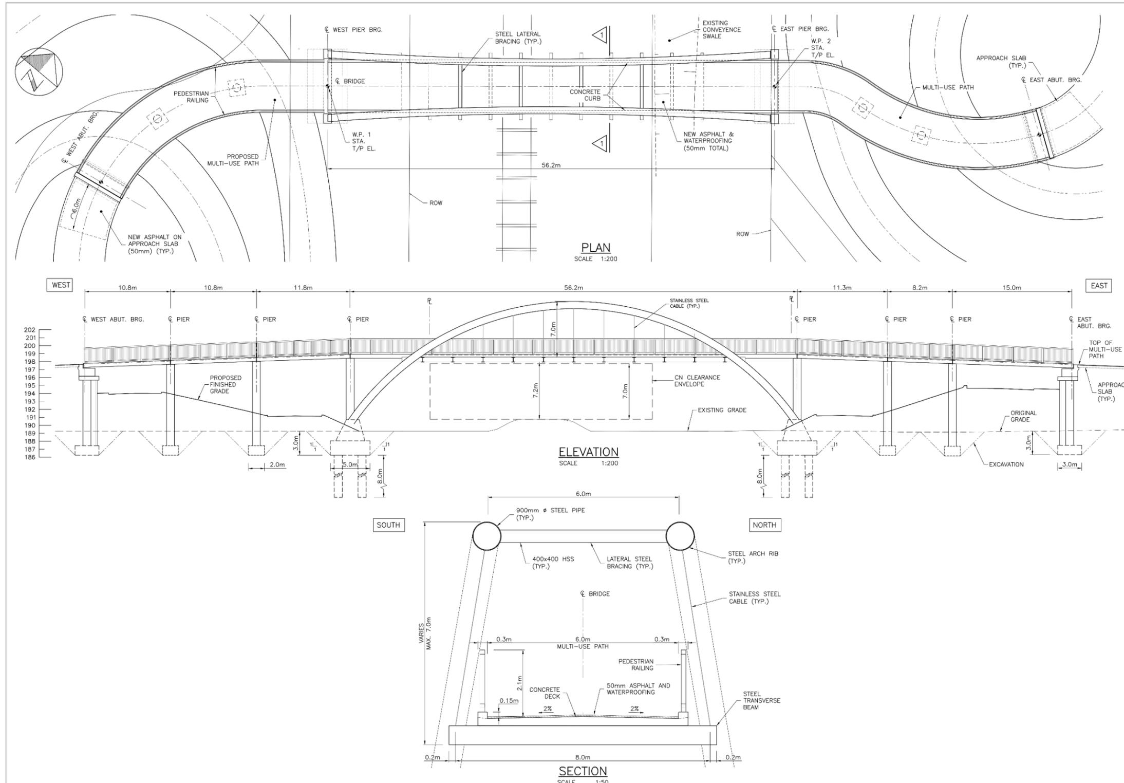
Figure 4-12: Alternative D2: Full Height Arch Bridge with Hanger Cables with Alternative Option 2, 3 or 4
