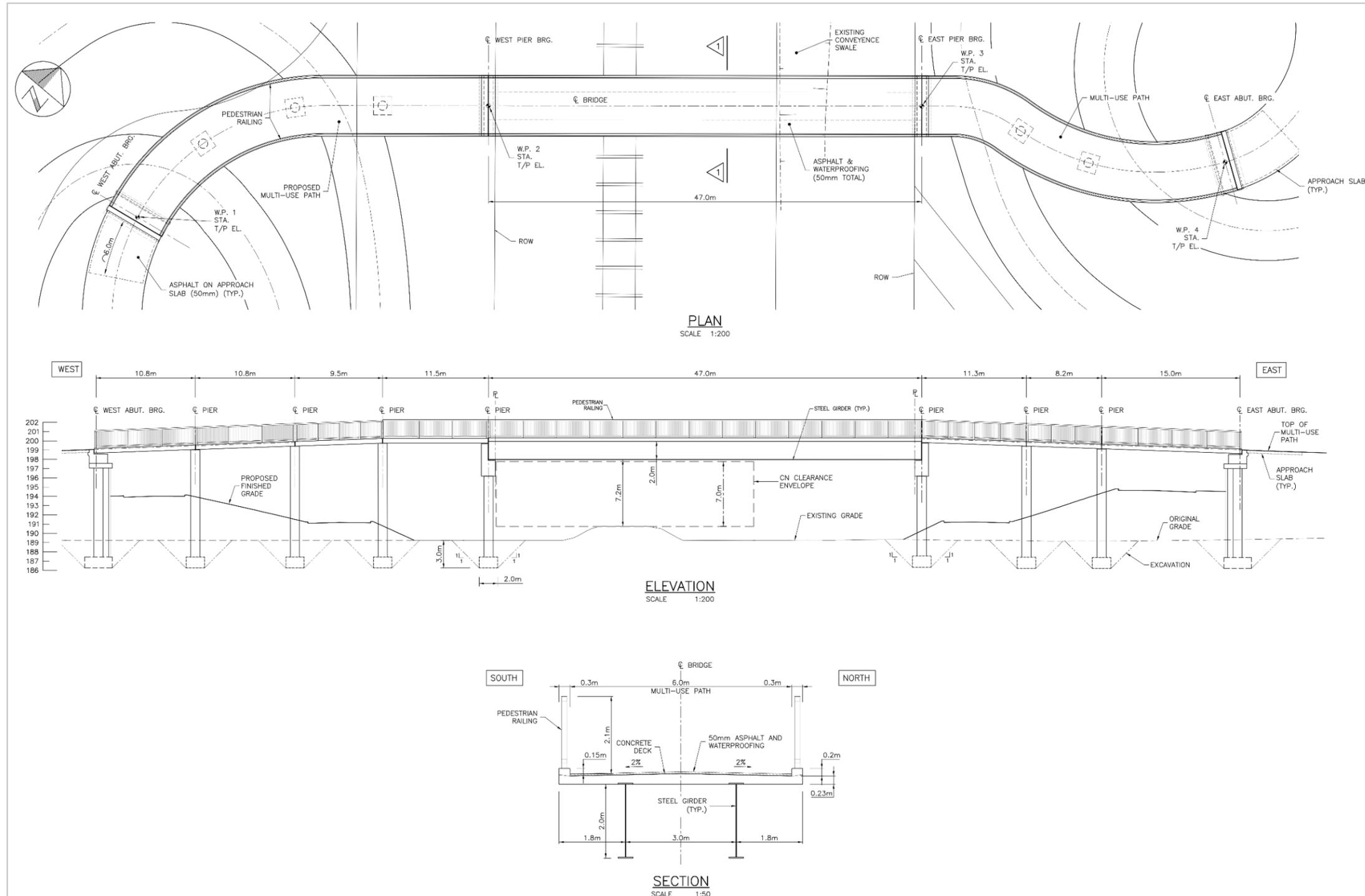
Figure 4-8: Alternative B2: Girder Bridge with Approach Alternative 2, 3 or 4
