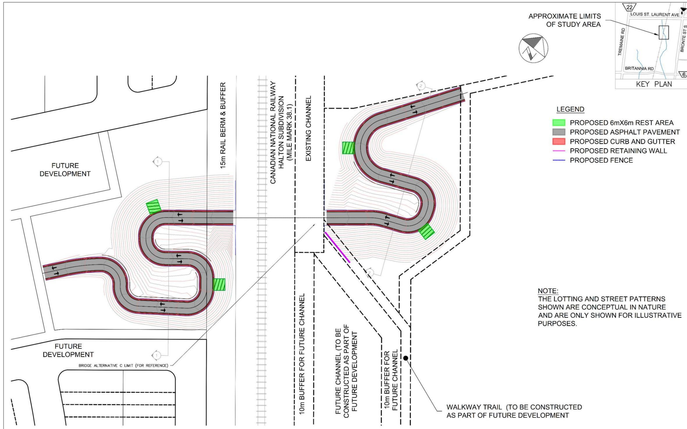
Figure 4-3: Bridge Approach Alternative 3 - Undulating Approach
