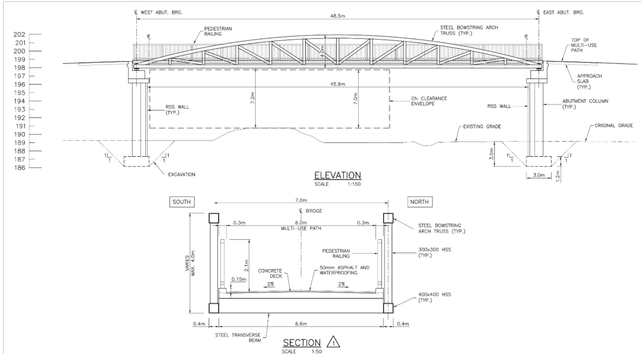
Figure 4-7: Alternative B1: Girder Bridge with Approach Alternative 1
