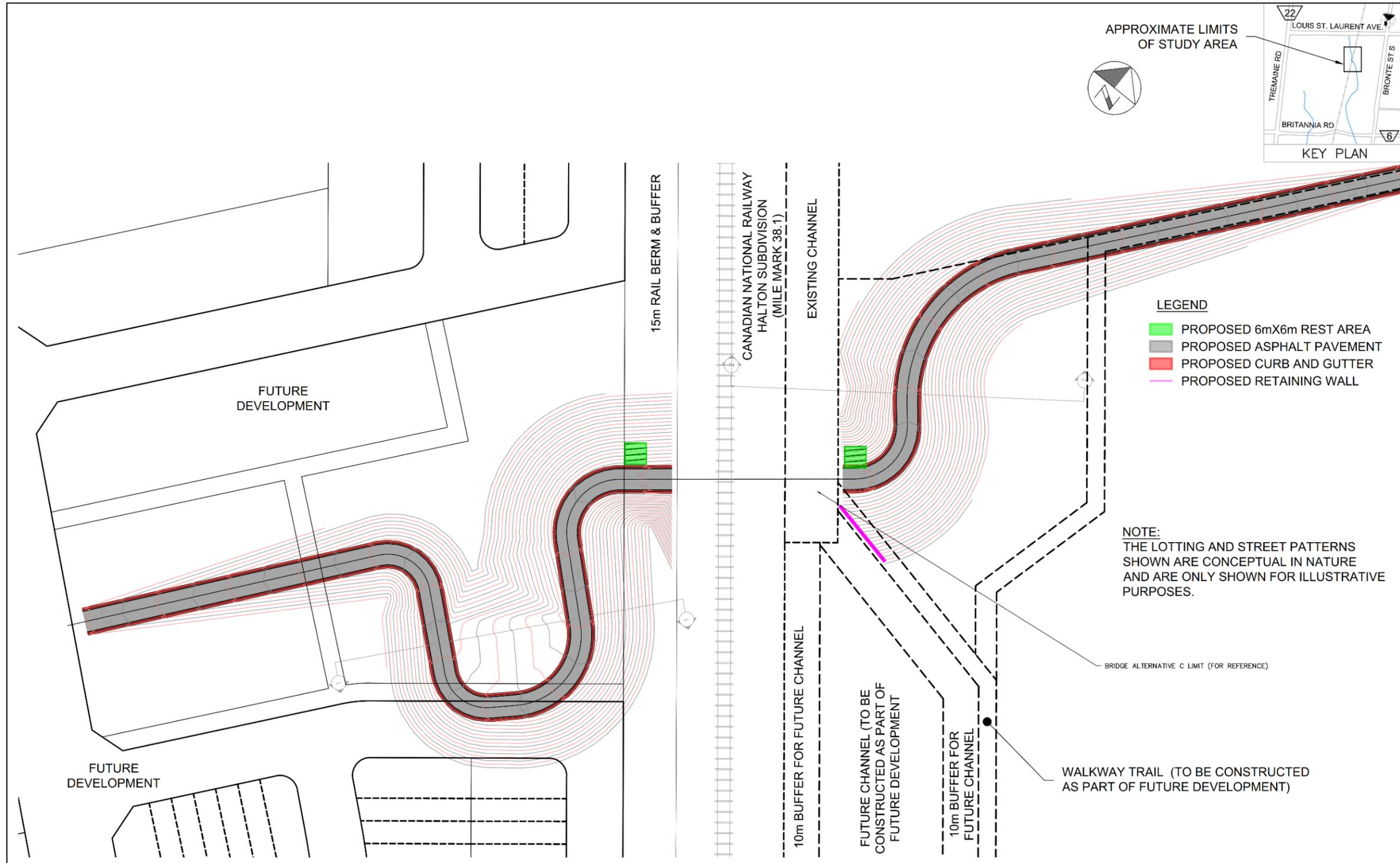
Figure 4-5: Bridge Structure Alternative A1: Bowstring Truss Bridge with Approach Alternative 1
