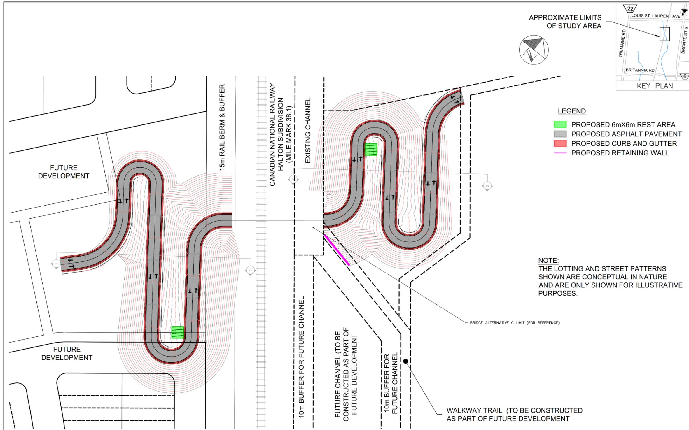
Figure 4-4: Bridge Approach Alternative 4 - Ramp Approach
