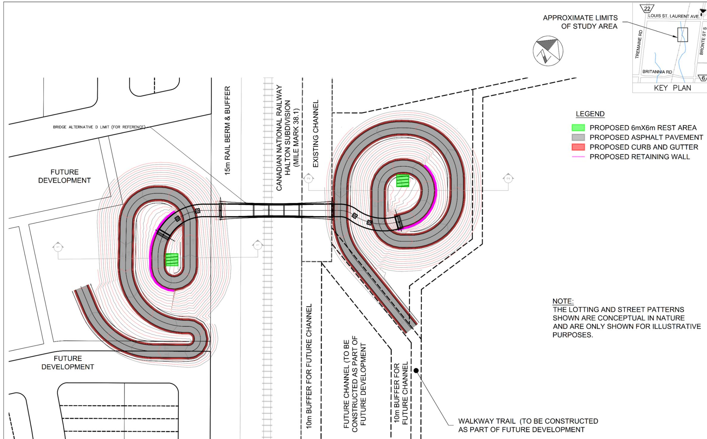
Figure 4-2: Bridge Approach Alternative 2 - "S" Shaped Approach
