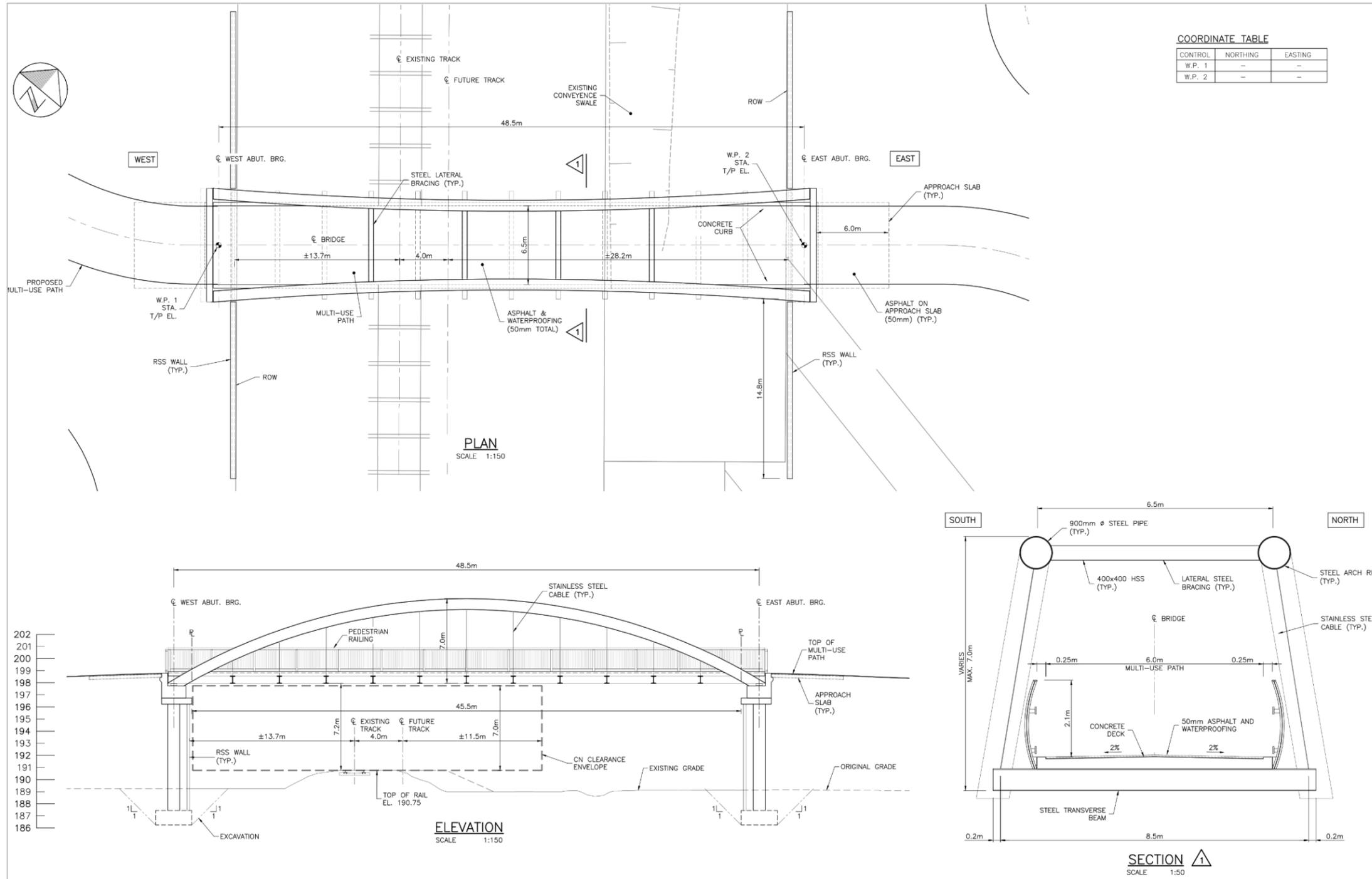
Figure 4-11: Alternative D1: Full Height Arch Bridge with Hanger Cables with Alternative Option 1
